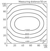
Illuminance based on the example of two 15 W luminaires with CDP screen that are swiveled at an angle of 90° (Distance between the two luminaire heads approx. 90 cm)
