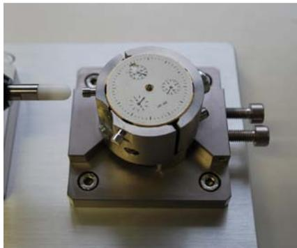
2. Move the mobile table and rest the tip of the sensor against a push-button.
